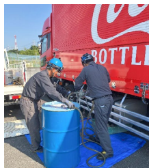
Diesel removal operation for switching to alternative fuel
