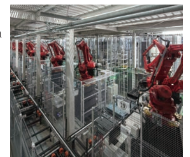
Saitama Mega DC automated picking system
