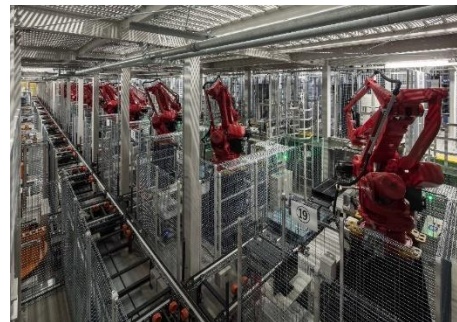
Saitama Mega DC and automated picking system
