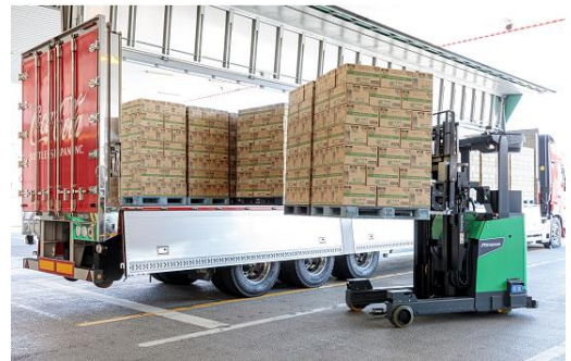
Automatic forklifts for loading and unloading trucks
